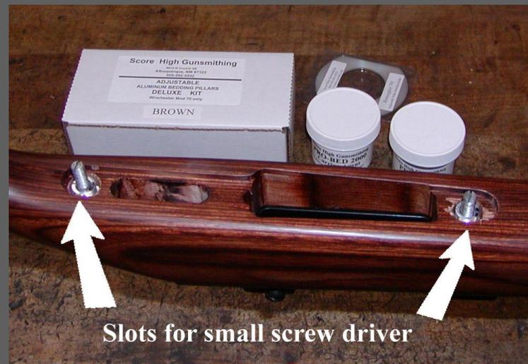
Holding the barrel and action firmly in the stock, use a small screw driver to rotate the adjustment post of each pillar so that it is flush or slightly higher than the level of the stock.
