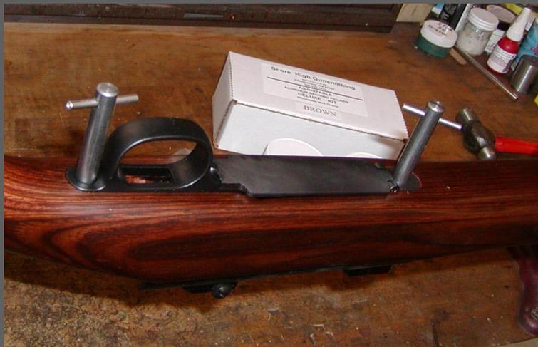
With the magazine box in place, slide the trigger guard over the retaining screws and tighten it down with the "T" handles. The "T" handles should tighten firmly, there should not be any mushy feeling to them at all.
