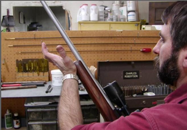
This can be easily tested by gently rapping on the bottom of the forend and listening for the sound of the forend striking the barrel. Hopefully it won't.
