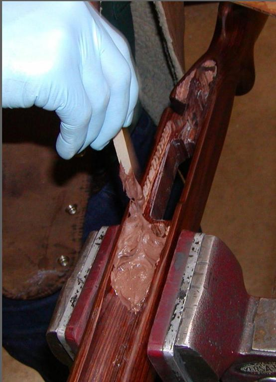
First apply the epoxy compound into the front pillar hole and then completely fill the lug area. The majority of the epoxy should lay flat on the bottom so that when the barreled action is inserted into the stock, the very bottom of the action will come into contact with the epoxy first and the epoxy will then flow up around the receiver eliminating any air bubbles.
