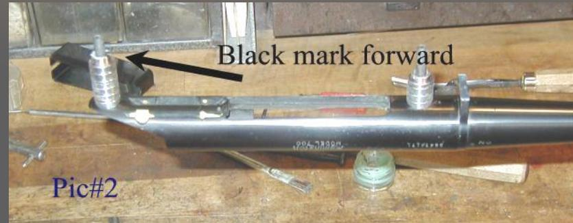
Each pillar has a threaded post with a screw driver slot used for adjusting the pillars length. There is one short pillar used for the front guard screw and one long pillar used at the rear. Each threaded post is cut at 2.5 degrees to match the angle of the trigger guard. You will find a black mark on one of the screw driver slots. This black mark should always be toward the muzzle.
