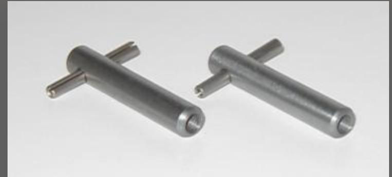
Each kit also contains two “T” handles that hold the assembly together during the epoxy process
