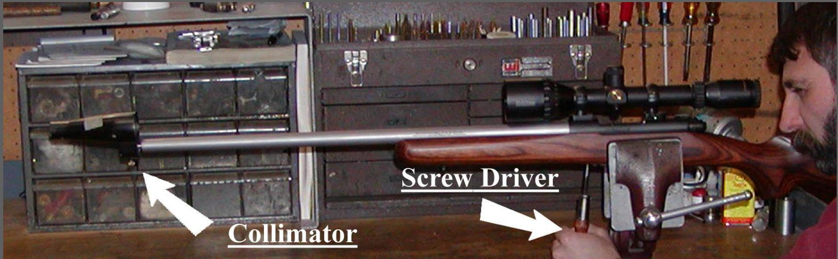
You should not be able to detect any change whatsoever in the collimator's view. Any change in that view illustrates how stresses are changing under the changing load of the guard screws. If there are no stresses there are no changes.
