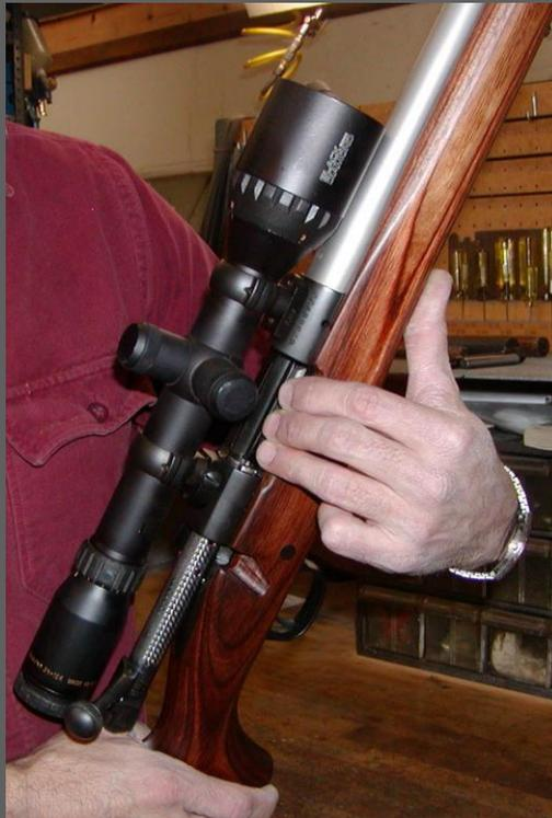
Placing one or more of your finger tips on both the stock and metal at the rear tang and then the ejection port while loosening and tightening the front and rear screws you can detect any stress by feeling for a change in the relationship of stock and metal. The middle screw should not be tightened.
