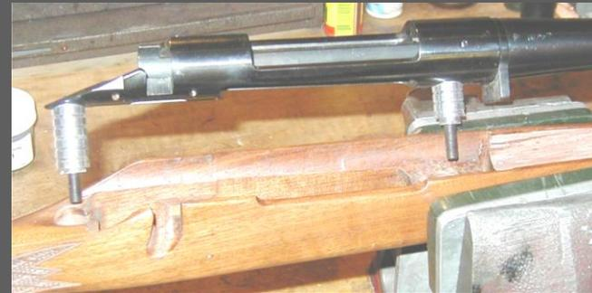
In having the pillars attached to the action, two very important things happen. First the pillars cannot get out of position during the epoxy bedding process. Second and most important of all, the pre-contoured pillars are allowed to seek their own path off the action to absolutely guarantee 100% contact with action after the epoxy cures. All this equals “ZERO” stress.
