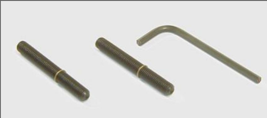
There are two double ended screws that are used to attach the pillars to the action. One end is  $\frac{1}{4}$  X 32 and it screws into the action. The other end is  $\frac{1}{4}$  X 28, has a hex key recess and screws into the “T” handles.
