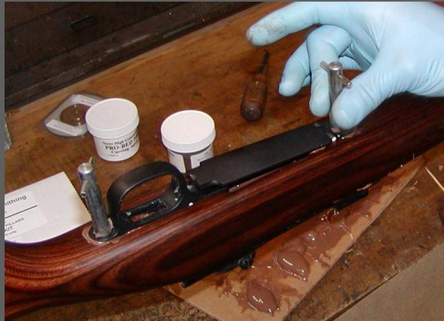
It is also very important that the “T” handles are not over tightened! It is very easy to induce stress in the assembly by over tightening. Once you feel the trigger guard come into contact with the pillars stop and back off the “T” handles just a tiny bit.
